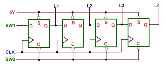
Figure 1. 4-bit shift register.
