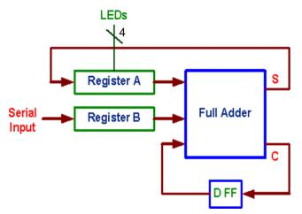
Figure 4. Block diagram of a serial adder.
