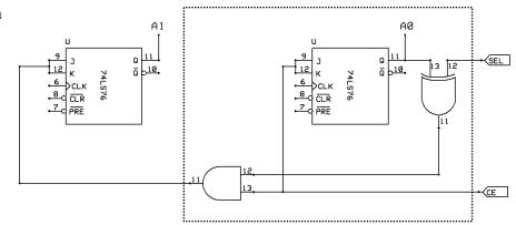
The circuit inside the dotted block (flip-flop A0 and the two gates) is the iterative module. If the counter had more than two flipflops, then each one, except the last (at the left), would look exactly like A0's circuit. This would require that the wire from the SEL input be continued across the whole counter. Because this is only a 2-bit counter, the last flipflop, A1, doesn't need any gates since there is nothing to its left.
