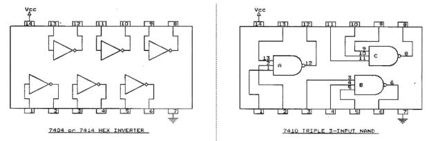
For each gate, draw the wiring diagram (including pin numbers) in your lab manual. As before, you do not have to redraw the 7493 counter for each wiring diagram. Just label the inputs of the gates with the appropriate Q output from the counter; i.e. QA for the inverter and QC, QB,QA for the NAND. For each gate, draw the waveforms of the msb (most significant input bit) and the output of the respective gate and verify that the output matches your truth table values from section 3.1.
