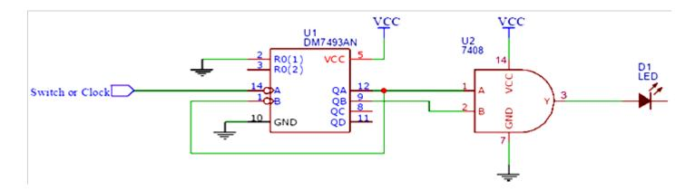
Connect QB and QA to two inputs of a 7408 AND gate. (Don't forget 5V and ground connections; pins 14 and 7. If you forget, the chip is inactive). Referring to the truth tables in 3.1, X = QB and Y = QA. Connect the clock A input of the counter (pin 14) to a pulser output. Connect QB, QA, and the output of the AND gate to LEDs and verify that the correct outputs are produced by referring to the truth table below (or your answer to part 3.1).
