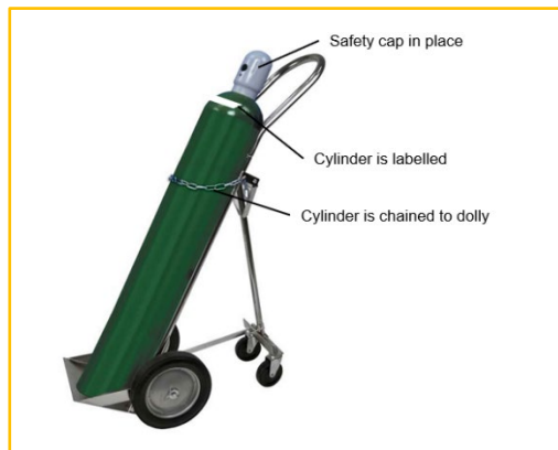
Figure 6-2: Proper gas cylinder transport.
